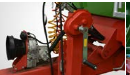
The tipping device with its own pump and oil tank allows coupling with tractors with smaller oil requirements.
