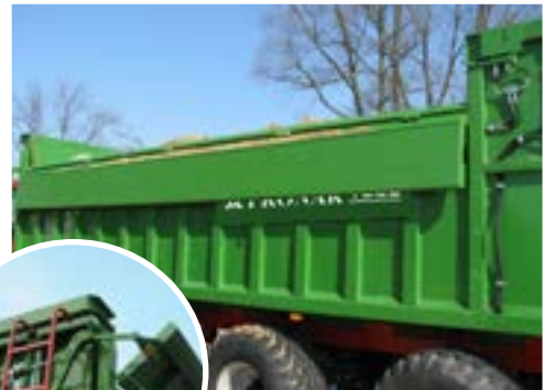
The optional hydraulic side wall enables loading from lower machines.
