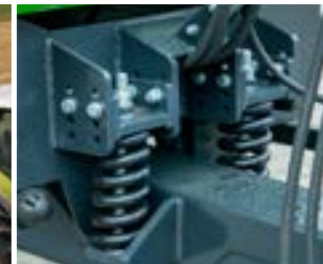
Universal drawbar damped by steel springs, height adjustable for connection to the lower or upper hitch of the tractor.
