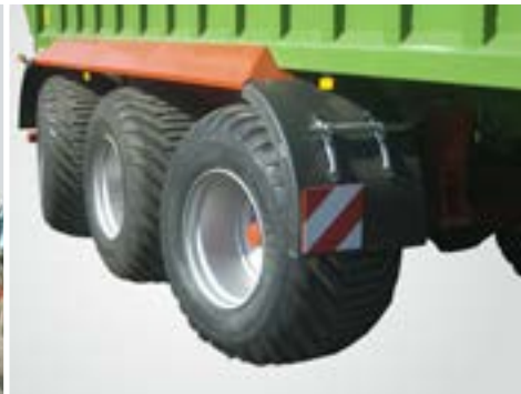
Thanks to the front and rear steering axles, the trailer follows the tractor very well and the tires are less worn.
