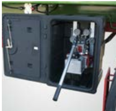
Adjusting the pressure in the active control system takes little time, but gives the possibility of very smooth manoeuvring in the curves.
