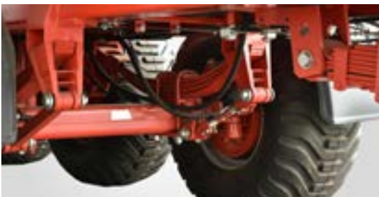
1. and 3. Trailing axle improves driving characteristics, increases driving safety and reduces Tire wear.
