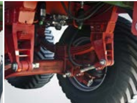
Parabolic suspension as standard. Hydraulic suspension can also be selected as an option.
