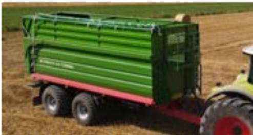
Attachments 600 mm | 23.6" from sheet metal 2 mm | 5/64" with the perforated viewing window and PLEXI pane increase the loading volume of the trailer up to 34,8 m³ | 1229ft³.
